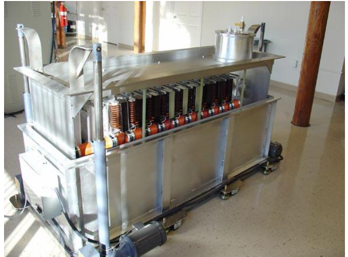
Fig. 8. Picture of the Unipolar Marx with Magnetic Assist
