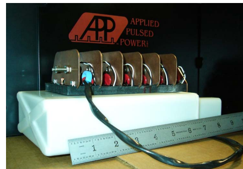
Fig 2. 24 kV, 10 kA Switch installed on 0.15 \mu\text{F} Capacitor
